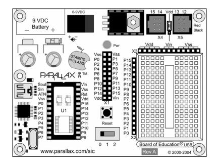
**Power Supply Clip and Barrel Jack (top left):** The 9 V battery clip and the barrel jack are positioned so that they cannot be accidentally used at the same time. For the jack we recommend our 9 VDC V 300 mA supply, # 750-00008.
